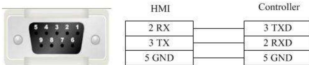
▪ Modbus RTU Server series RS485-2 cable
